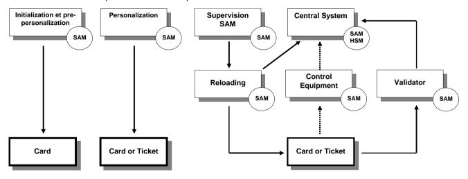
Actually, the secure modules (SAM) are also microprocessor smart cards. The information that they contain are protected by SAM system secret keys (called "SAM keys"). For on-line operations such as remote loading, an HSM (Hardware Security Module) may be used instead of a SAM.
