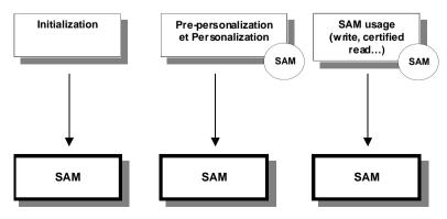
Furthermore, in order to increase the system security, the modules are not all identical. A module only contains the keys necessary for its use, each of the key being limited only to the necessary actions (ciphering, personalization, etc.).
